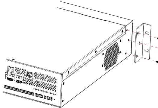
2. Install the matrix in the rack by using the mounting screws to affix the matrix to the rack.
