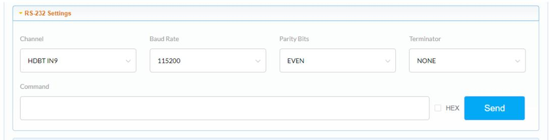
This section allows users to set parameters for RS-232 routing (from matrix LAN port to HDBT and NHD ports).
