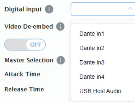
**Note:** The matrix is equipped with a built-in USB audio speaker, when the matrix is used for conferencing through remote conferencing software, and the laptop can select the matrix USB audio speaker, this source is from the conferencing software. When select the USB Host Audio, it will be mixed to output from the output channels users selected.
