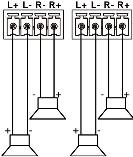
2) Connection with 2 x 30watts 8Ω speakers, or 2 x 50watts 4Ω speakers
